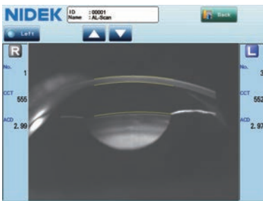
Sectional lens image (Scheimpflug image)
